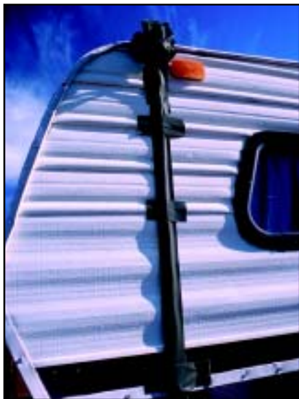
Figure 3 —It was such a tight fit on the four-wheel-drive road through the piñon pine forest to Kanab Point that the trees would rip away anything that wasn't taped against the camper body. Covered up here is the coax feed for the VHF/UHF antenna mount. Even with all the tape and just creeping along, we lost half the railing on the roof.
