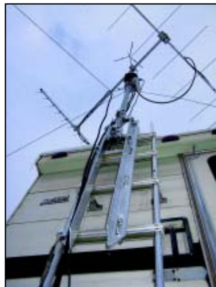
Figure 1—Gap's "Quick Tilt" ground mount was a better bet for the 60-pound antenna and rotator array since its longer legs enabled me to spread the load over four steps of my camper's ladder.
