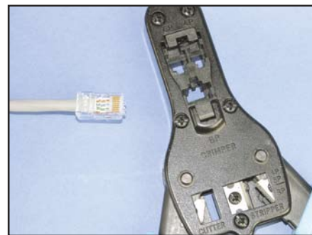
Figure 3 — Wires arranged and inserted in the RJ-45 connector ready to crimp.
